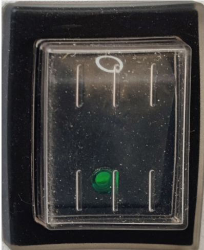
Fig. 18: Power switch with splash protection cap
